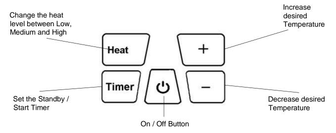
Please note the unit must be turned on using the power switch before use
